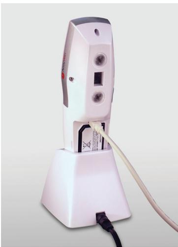
Plug the USB cable into the AV300's USB port, which is above the battery, and place the AV300 in its charging cradle. Plug the other end of the USB cable into your PC's USB port. Then start the AV300 PC application, which begins looking for the attached AV300. **Be sure to leave the AV300 in its charging cradle while it's plugged into the computer.** The AV300 fits in the cradle with the battery cover removed.
