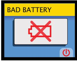
The AV300 checks the battery periodically to ensure that the battery is in good condition. If a **Bad Battery** warning appears, the AV300 does not function and you must replace the battery. Turn the device off by pressing the right circular Power button. The unit will turn off automatically in 30 seconds once a bad battery is detected.
