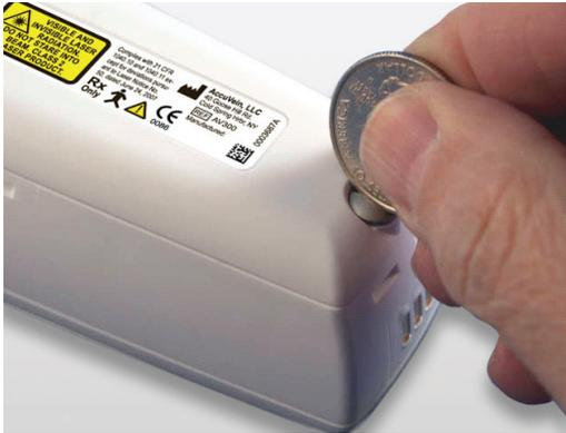
The BA300 battery can easily be removed from the battery compartment or inserted, as its shape matches the AV300 battery compartment.
