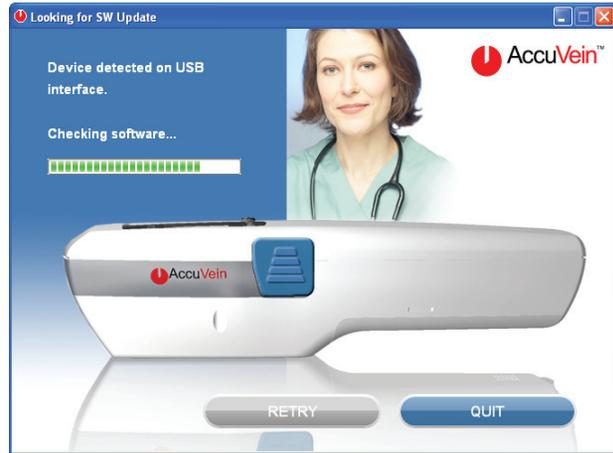
**If the PC application can't find the AV300**, the following screen appears. Verify the USB connections and that the AV300 is turned on, and click Retry to try connecting again.
