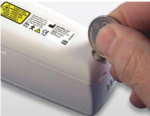
Once the AV300 PC Application is installed on your computer, connect the AV300 to the computer using the USB cable included with the device. To begin, remove the AV300's battery cover at the rear of the device. Use a screwdriver or small coin to loosen the screw holding the cover in place.
