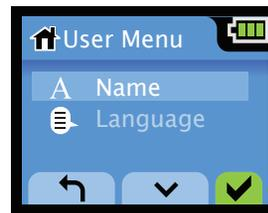
**To label an AV300,** go to the **Settings > User > Name** screen. From this screen, press the up/down arrows to select a character, press the green check mark to move to the next character, and continue until you have entered the entire name. Use the left/right arrows to scroll through and change existing characters. When you’re done, select **SAVE** and press the green check mark to save the name. Select **CLEAR** to clear the AV300 name.
