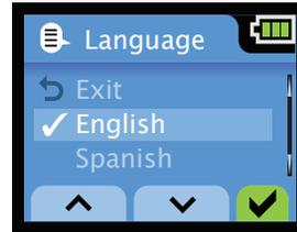
**To exit the menu without changing the setting,** scroll to the Exit item in the list and press the green check mark button, or press the Blue side button to escape the menu.
